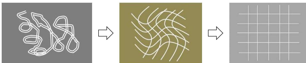
Figure 1.3 Schematic diagrams of crystal structures of glassy-carbon (left), glassy-graphene (middle) and graphene (right), respectively. The lines in the images denote distribution of carbon atoms. The images were cited from Ref. 24.
