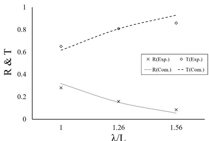
**Fig 4** Computational and experimental R & T, as a function of wavelength divided by ice length.
