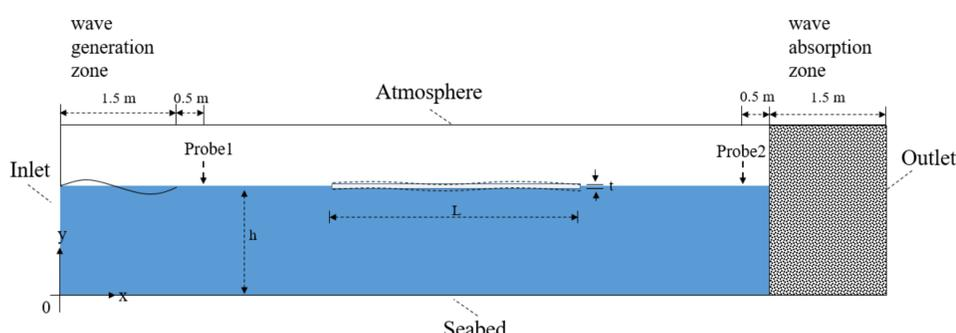
**Fig 2** Schematic of the case: an ice sheet is floating on the water surface and subjected to incoming waves.
