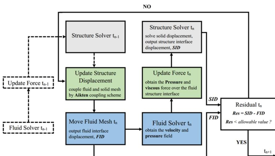
**Fig 1** Flowchart of the FSI procedure.
