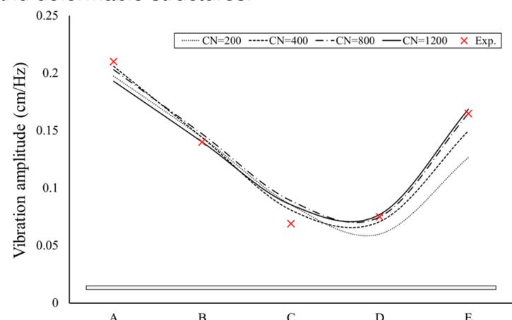
**Fig 3** Vibration amplitude at different locations of the ice sheet, calculated with a range of solid cell number (CN).
