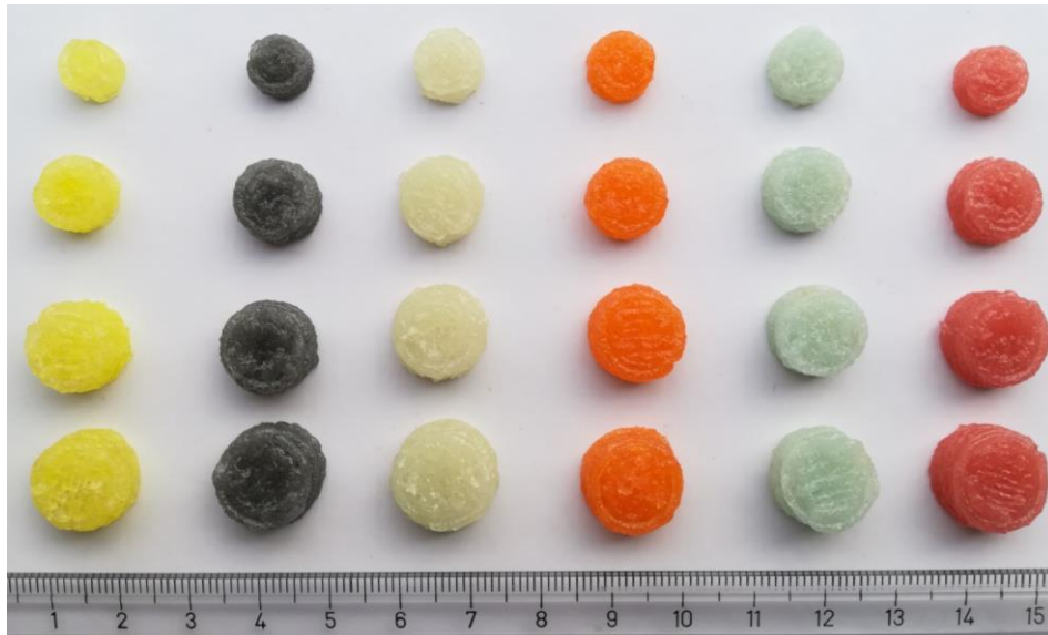
264 265 Figure 2. Chewable printlets in different flavours/colour and doses. From left to right: 266 Lemon/yellow, Coconut/ black, Banana/light green, Orange/orange, Raspberry/light blue, 267 Strawberry/red. From top to bottom: 50mg, 100 mg, 150 mg and 200 mg. Units are cm.
