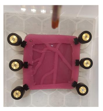
Fig. 4. Photograph of the placenta phantom from above to show the positions of the posts to maintain the position of the phantom.
