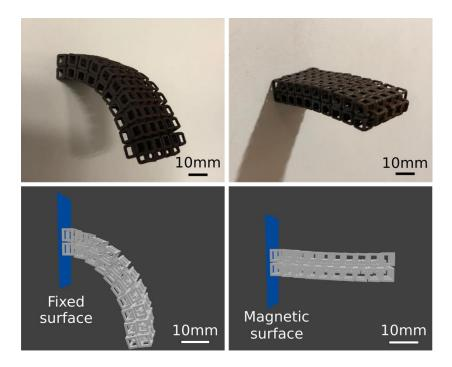
Figure 4: Experimental (a, b) and simulated (c, d) post-processed Fe-mails, in the unactuated (a, c) and actuated (b, d) states.
