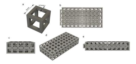
Figure 1: (a) Geometry of a cube link, (b) top view, c) end view, d) perspective view and e) side view of the CAD chainmail.
