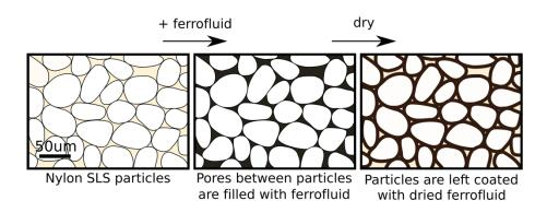
Figure 2: Schematic cross-section of the post-processing method, where SLS prints were dipped in ferrofluid and then dried. The process deposits magnetic nanoparticles in the form of dried ferrofluid throughout the porous material.
