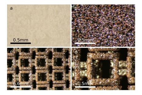
Figure 3: Optical micrographs of a) Unprocessed SLS print b) Post-processed SLS print c) Post-processed Fe-mail d) Post-processed Fe-mail link.
