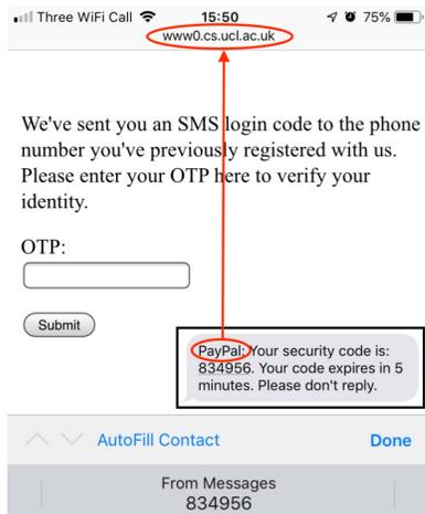
Figure 2: Screenshot: Security Code AutoFill suggested to fill a security code into an unrelated website. The SMS exposes a discrepancy between the SMS content and website.
