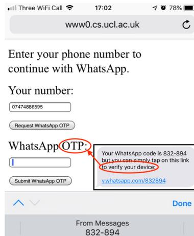
Figure 3: Screenshot: Security Code AutoFill suggested to fill a security code into an unrelated website. The SMS exposes a discrepancy between the SMS content and website.
