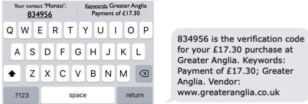
(a) Design sketch of alternative autofill suggestion for an online payment. Sketch of corresponding SMS shown in fig. 5b. (b) Design sketch of security code sent via SMS with additional keywords indentifying salient context information.
