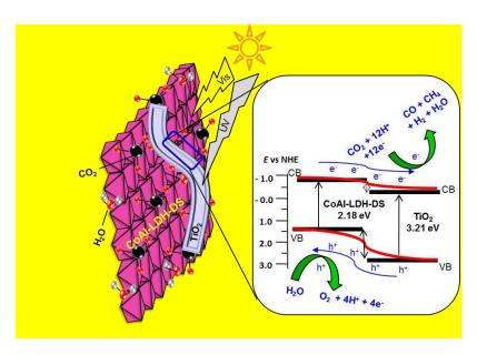
**Scheme 2.** Proposed mechanism of CO<sub>2</sub> photocatalytic reduction over CoAl-LDH-DS@TiO<sub>2</sub>-NT heterojunction nanocomposite.
