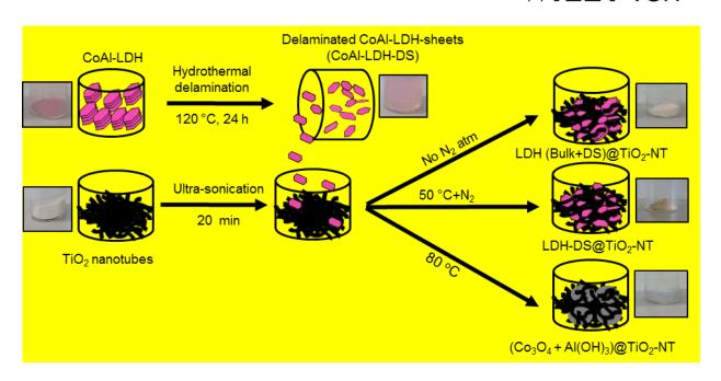
**Scheme 1.** Schematic of CoAl-LDH@TiO<sub>2</sub> nanocomposite synthesis.
