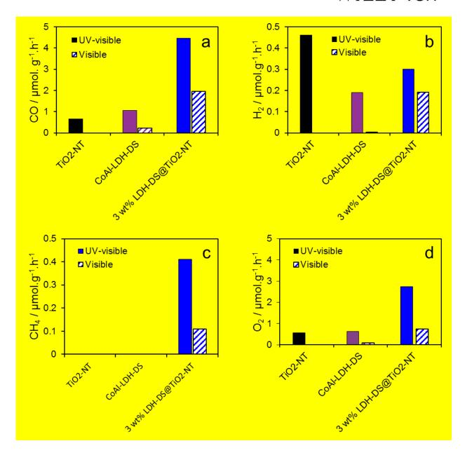
**Figure 5.** Comparison of (a) CH<sub>4</sub>, (b) CO, (c) H<sub>2</sub> and (d) O<sub>2</sub> mass-normalized productivity averaged over the first 4 h of aqueous phase CO<sub>2</sub> photoreduction over 3 wt% LDH-DS@TiO<sub>2</sub>-NT nanocomposite, and CoAl-LDH-DS and TiO<sub>2</sub>-NT references under UV-Vis versus visible only light irradiation.
