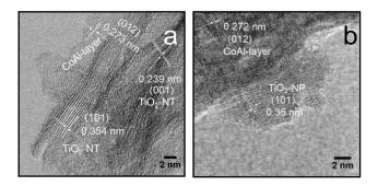
Figure 3. High resolution TEM images (a) 3 wt% LDH-DS@TiO<sub>2</sub>-NT, and (b) LDH-DS@TiO<sub>2</sub>-NP nanocomposites.
