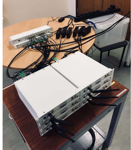
Fig. 6. USRP array setup for the MIMO-SEFDM precoding system.
