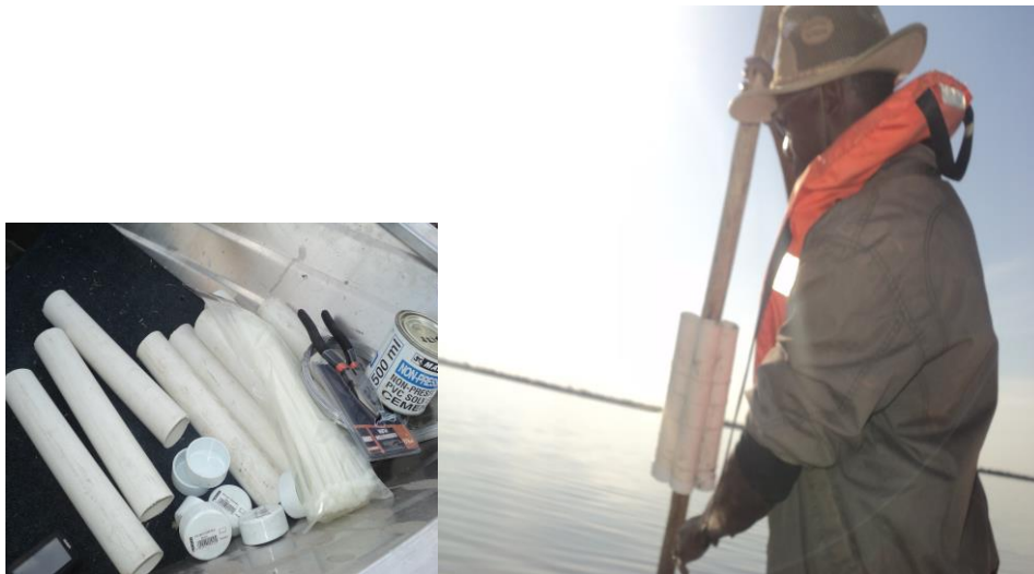
Figure 5.6: Sediment traps made from PVC pipes tied to a 3m pole. (Photographs: Author's own)
