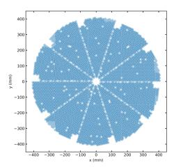
**Figure 2.** A single DESI tile, showing the arrangement of fibres in the focal plane, split into 10 petals. The blue circles indicate the patrol area of each fibre. The holes within each petal are the locations of the fiducials, which provide a light source for the fibre view camera to calibrate the placement of the fibre positioners.
