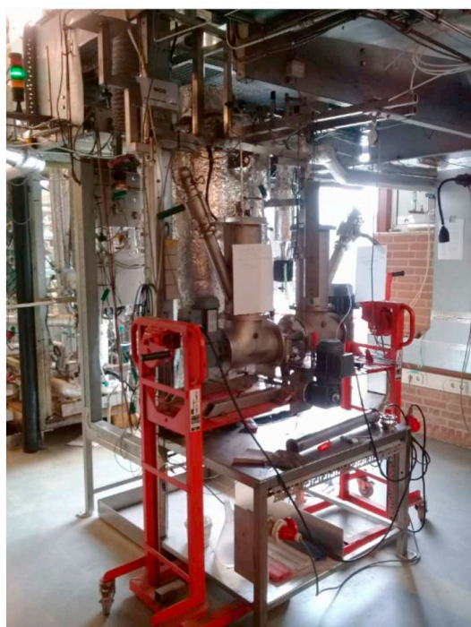
Fig. 1. Photography (left) and schematic diagram (right) of fluidized-bed reactor (ECN).
