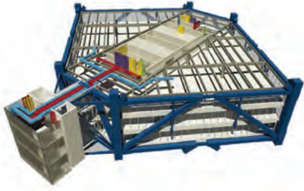
Figure 7. 3D Digital Prototype testing architectural decisions and the mechanical services strategy. A holistic digital prototype, built and maintained by the London-based design team, ensured speed and quality of design development. (Source: Rogers Stirk Harbour+Partners) 图7: 三维数字样机测试建筑的决定和机械服务策略。为确保开发的质量和数据的准确, 伦敦的设计团队建立并维护了全面数字样机。(来源: Rogers Stirk Harbour+Partners)
