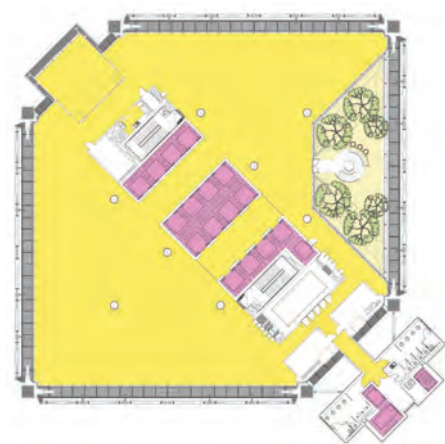
Figure 2. Typical floor plan showing the hexagonal trussed tube with internal columns. The soft core and umbilical core are not part of the structural stability system but supply all services. Sky Gardens occur every 9 levels. (Source: Rogers Stirk Harbour+Partners) 图2. 典型的建筑平面图，展示了有内柱的六桁架筒。软核和脐带中心对系统的稳定性虽无作用，却能提供所有服务。每9层建有一个有空花园。(来源: Rogers Stirk Harbour+Partners)
