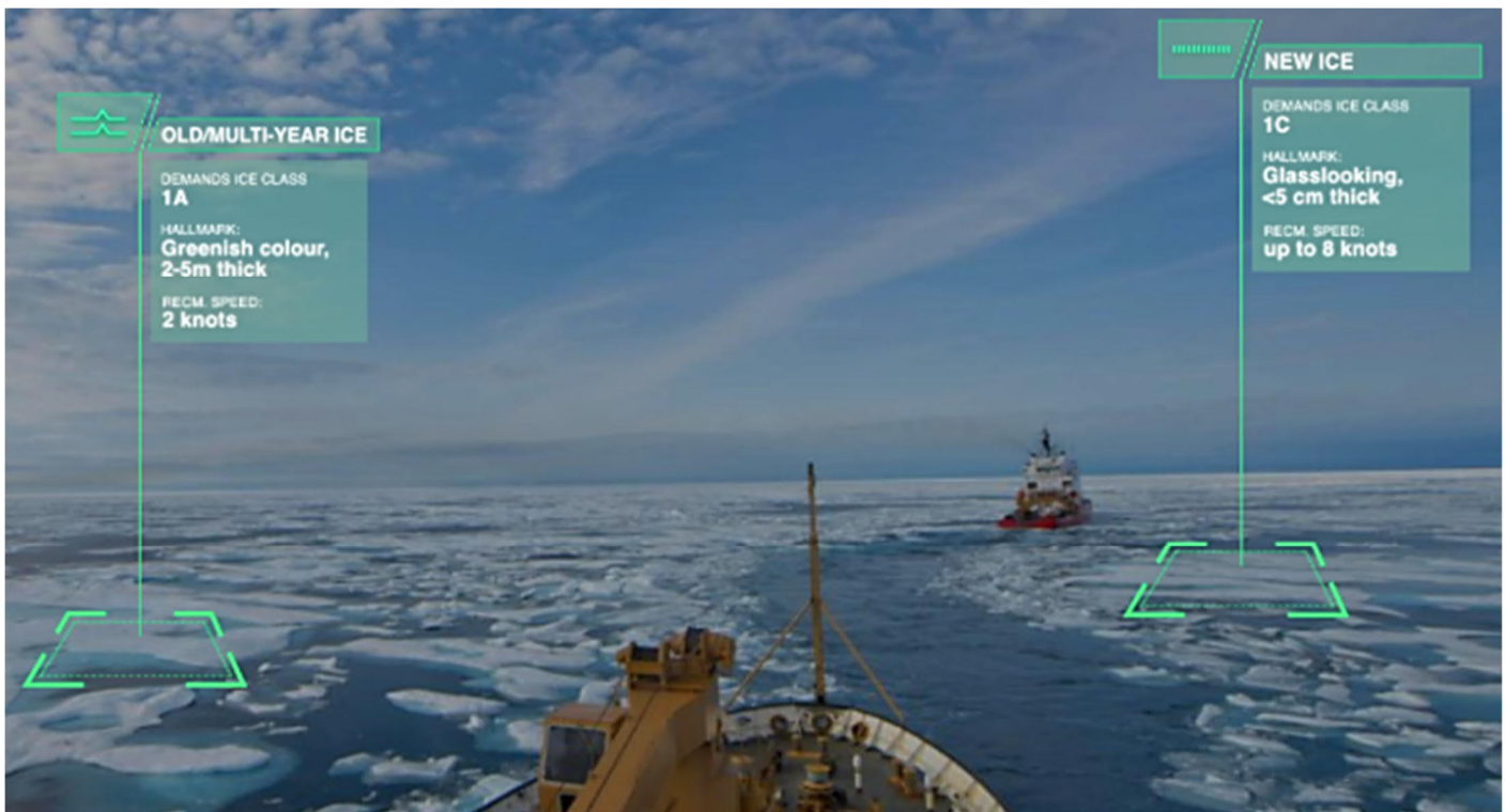
Figure 3: Example of how AR technology could be applied for an improved situation awareness in Arctic ship operations. ©Amalie Albert
