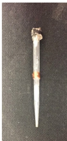
Figure 2. The pipettes were filled with \text{LaF}_3:\text{Tb}^{3+} or \text{Y}_2\text{O}_3:\text{Eu}^{3+} NP's.
