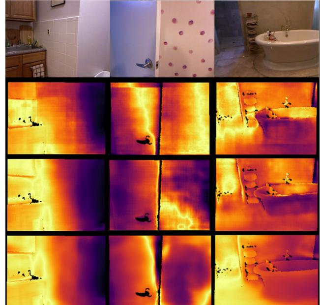
**Fig. 9** Input image and errors for three different models. Top row: input image. Second row: Transposed. Third row: Depth-to-Space. Fourth row: Bilinear additive upsampling. We observe that our proposed upsampling method produces smoother results with less artifacts.
