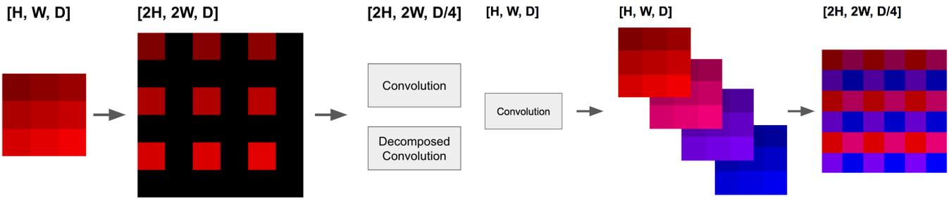
**Fig. 2** Visual illustration of (Decomposed) Transposed Convolution. The resolution is increased by interleaving the features with zeros. Afterwards either a normal or decomposed convolution is applied which reduces the number of channels by a factor 4.
