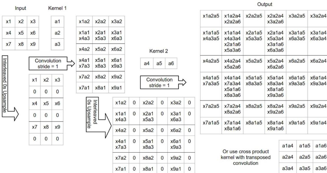
**Fig. 5** Spatial dependency for the outputs of a Decomposed Transposed Convolution with kernel size 3 and stride 2.
