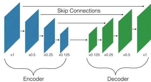
**Fig. 1** General schematic architecture used for dense prediction problems. Typically, the resolution is reduced by a factor 2 in each of several encoder steps, after which they are upsampled by a factor 2. In this illustration, the lowest resolution is  $0.125\times$  the input size.
