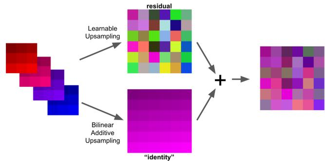
**Fig. 7** Visual illustration of our residual connection for upsampling layers. The “identity” layer is the sum of each four consecutive upsampled layers in order to get the desired number of channels and resolution.
