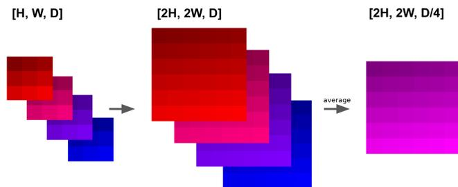
**Fig. 6** Visual illustration of our bilinear additive upsampling. We upsample all features and take the average over each four consecutive channels. For our upsampling layer this operation is followed by a convolution (not visualized).
