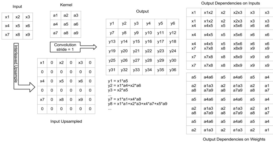
**Fig. 4** Spatial dependency for the outputs of a Transposed Convolution with kernel size 3 and stride 2.
