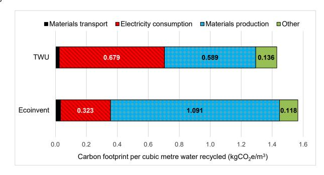
**Fig. 2**. Comparison and breakdown of subgroup contribution to the total OFWRP CF. The total aggregated CF values for the TWU and Ecoinvent analyses are 1.430 and 1.566 kgCO<sub>2</sub>e/m<sup>3</sup> respectively. For the categorical grouping of components, see Tables 1 and 2.
