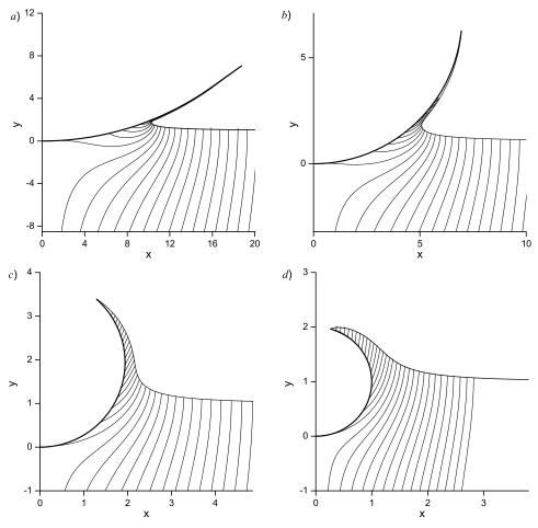
FIGURE 6. The flow configuration at the different expansion speeds: a) u = 27.6; b) u = 6.98; c) u = 1.94; d) u = 1.0.
