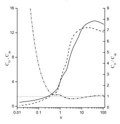
FIGURE 5. The Impact force coefficient on an expanding circular cylinder entering water with constant velocity:  $C_D$  in (46) (solid line);  $C_{dp}$  in (46) (dashed line); the ratio  $C_D/C_{dp}$  (dash-dotted line).
