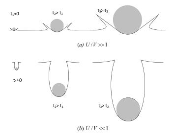
FIGURE 2. Flow development as time in progress for (a) fast expansion and (b) slow expansion.
