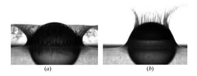
FIGURE 1. Impacting spheres with two different wettabilities at the same impact velocity: (a) hydrophobic sphere and (b) hydrophilic sphere. Adopted form Duez et al. (2007).
