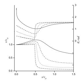
FIGURE 8. (a) Velocity magnitude along the free surface relative to the velocity at the jet tip,  $v/v_0$ , (lower set of the curves) and the angle of the velocity to the free surface,  $\theta$ , (upper set of the curves) for different expansion speeds: u = 20.2,  $\delta_O = 50^\circ$  (dashed-dot lines); u = 5.62,  $\delta_O = 90^\circ$  (dotted line); u = 2.09,  $\delta_O = 135^\circ$  (dashed line); u = 0.937,  $\delta_O = 167^\circ$  (solid line).
