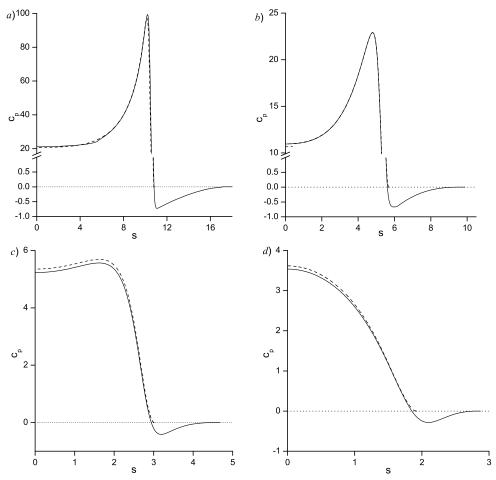
FIGURE 9. Pressure coefficient on the cylinder surface for the cases shown in figures 4 (dashed lines) and 6 (solid lines): (a) u = 27.17; b) u = 6.98; c) u = 1.94; d) u = 1.0.
