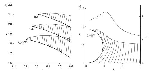
FIGURE 7. (a) the free surface shapes and the streamlines near the jet tip at the different angles of the wetted part of the cylinder  $\delta_O$ , and (b) free surface shape and velocity magnitude along the free surface at  $\delta_O = 167^\circ$  for u = 0.9365
