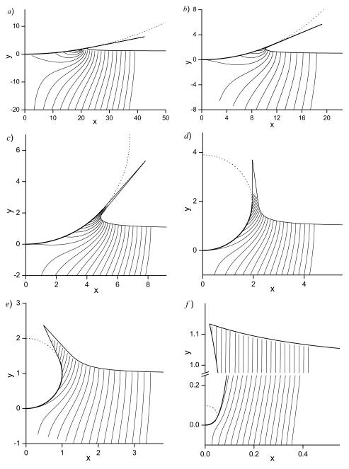
FIGURE 4. The free surface shape and streamlines for different expansion speeds of a circular cylinder: a) u = 109,  $b = 10^{-5}$ ; b) u = 27.6,  $b = 10^{-4}$ ; c) u = 6.98,  $b = 10^{-3}$ ; d) u = 1.94,  $b = 10^{-2}$ ; e) u = 1.0, b = 0.052; f) u = 0.0487, b = 4.0.
