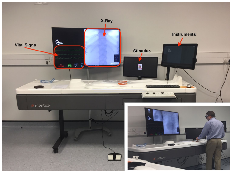
Fig. 1 Main image: Mentice VIST-Lab simulator, with the four AOIs identified. Bottom right: a participant during procedural performance, wearing eye tracking glasses connected to the portable recording device placed to the left on the simulator table and wearing the Empatica's E4 wristband on their wrist (hidden)
