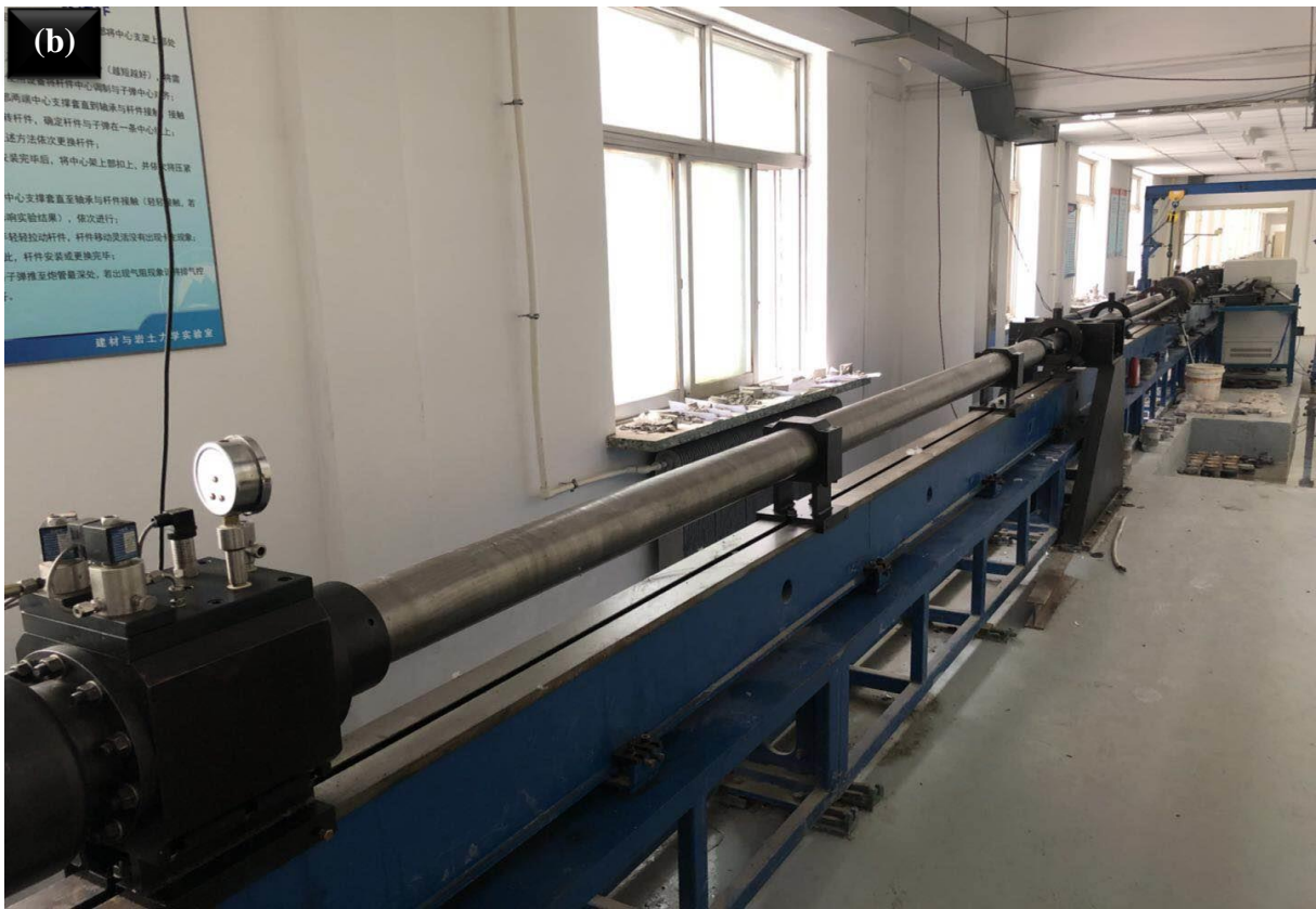
Fig. 2. Splitting Hopkinson pressure bar (SHPB) testing system: (a) schematic diagram; (b) picture
