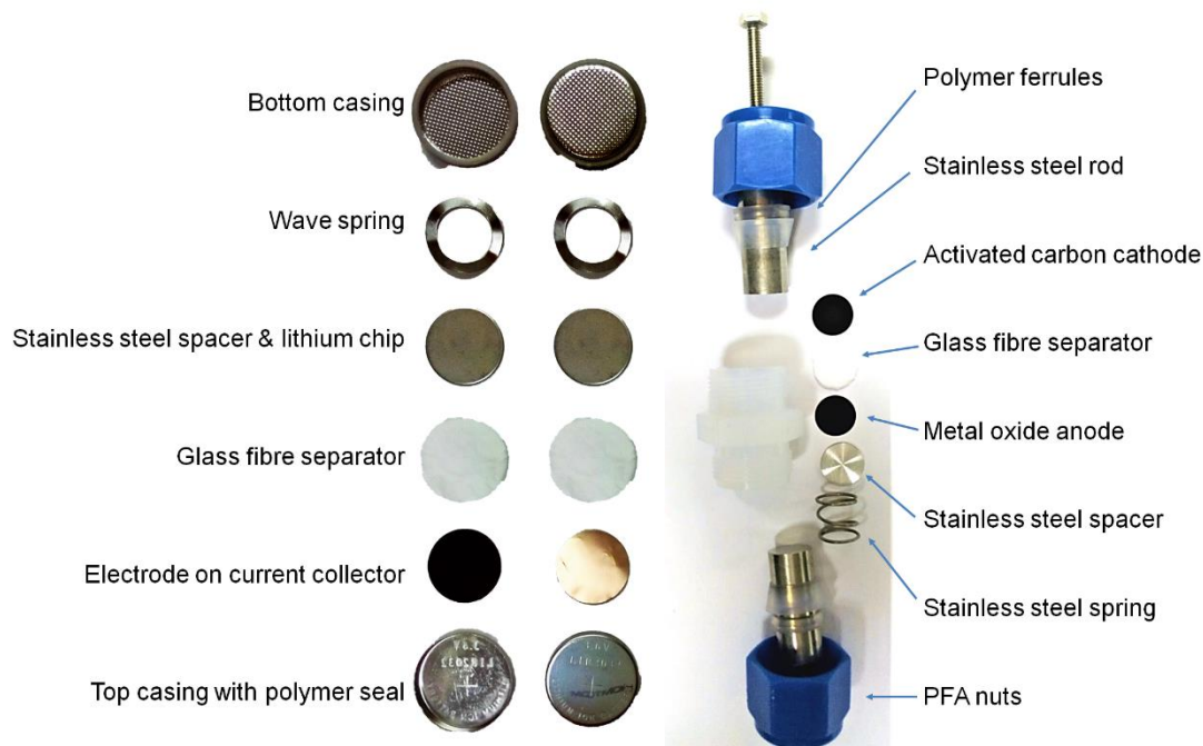
Figure 2-13: Photographs of the components of both coin cells and Swagelok-type cells.
