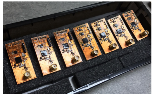
Fig. 2 The long range low power RF modules developed in UCL
