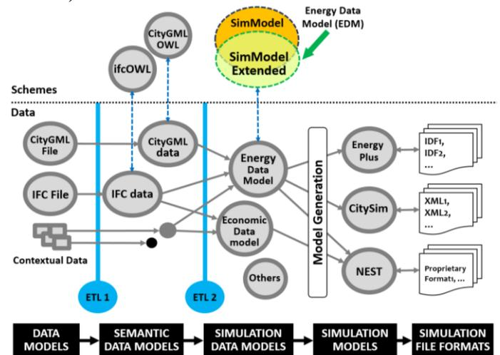
Figure 2. Overview of the data integration and transformation process in OptEEmAL platform. In this figure the process is exemplified for the case of EDM, EnergyPlus and CitySim tools.
