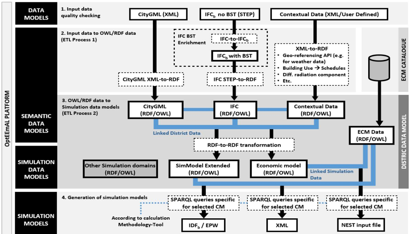
Figure 3. Data flow of the process to generate simulation models.
