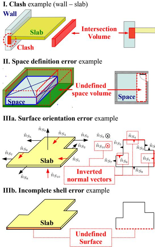
Figure 6: **I. Clash error:** A building slab intersects with a building wall. **II. Space definition error:** An internal building space is incorrectly defined leaving an undefined space-volume gap. **IIIa. Space orientation error:** Some of the outward normal vectors of a building B-rep are inverted. **IIIb. Incomplete shell error:** One or more surfaces in the B-rep are not defined.
