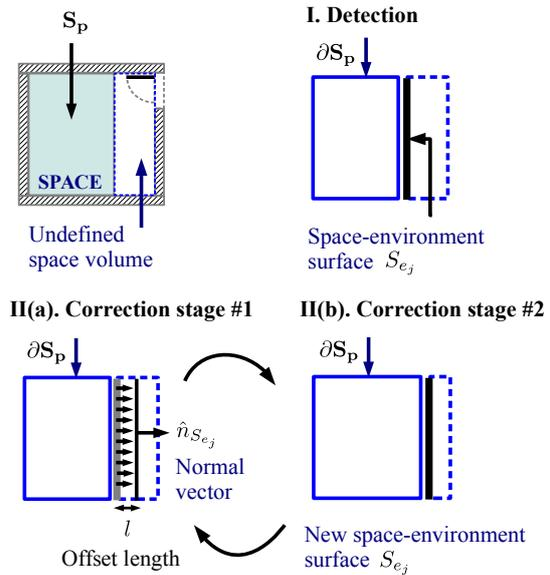
Figure 8: Space definition error detection and correction. **I. Detection:** Space environment surfaces are extracted. **II(a). Correction stage #1:** The internal space is inflated towards the normal vector of every space-environment surface, for offset length  $l$ . **II(b). Correction stage #2:** New space-environment surfaces are extracted after the inflation.
