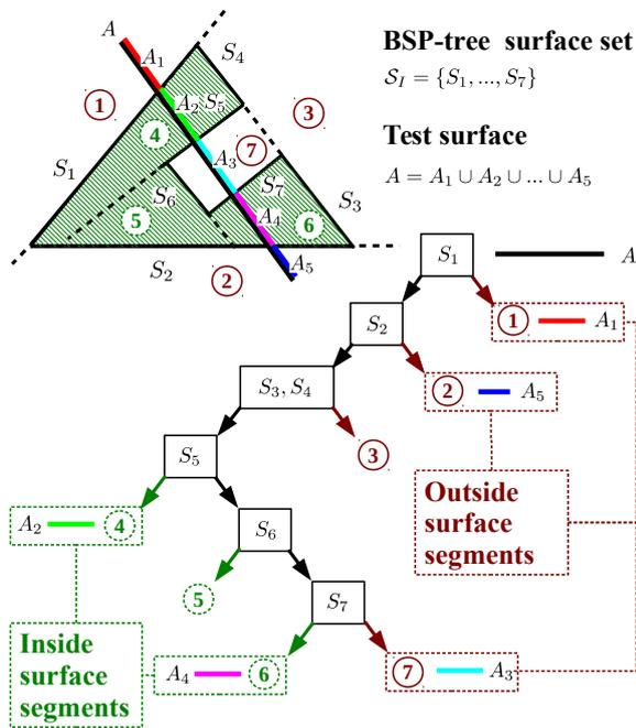
Figure 4: Demonstration of a filtering capabilities of a BSP-tree  $T_{S_I}$  on a test surface  $A$ .
