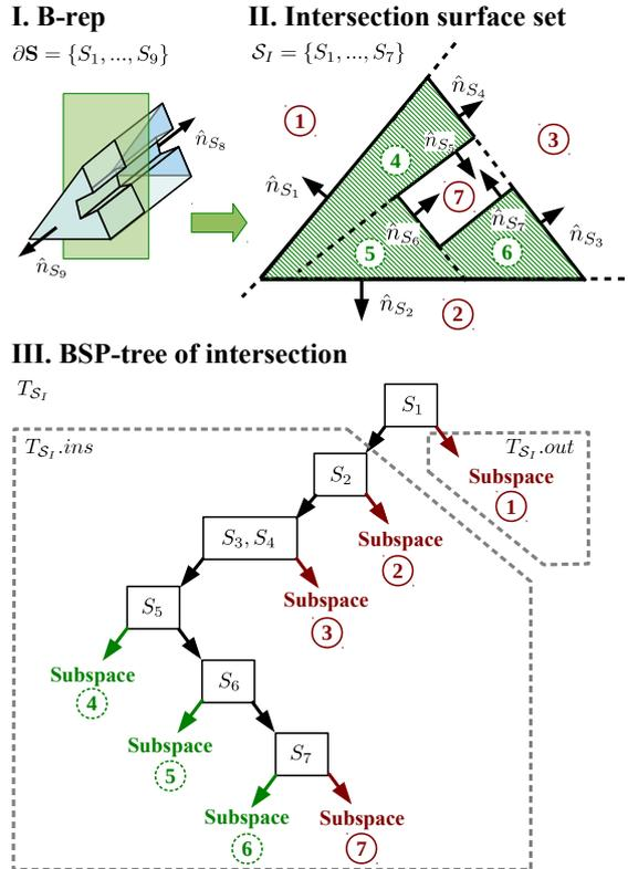
Figure 3: Example of a Binary Space Partitioning tree (BSP-tree)  $T_{S_I}$  of a surface set  $\mathcal{S}_I = \{S_1, \dots, S_7\}$  which is a subset of the B-rep  $\partial S$  of a building solid S.
