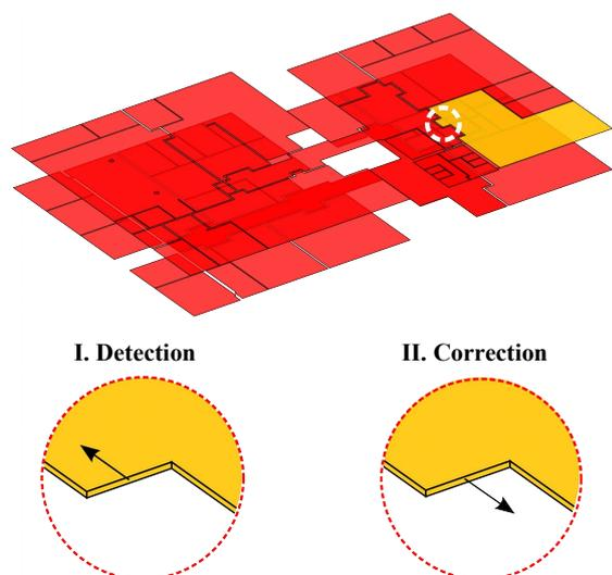
Figure 13: Surface orientation error example in CAR-TIF building: **detection (I)** and **correction (II)**.
