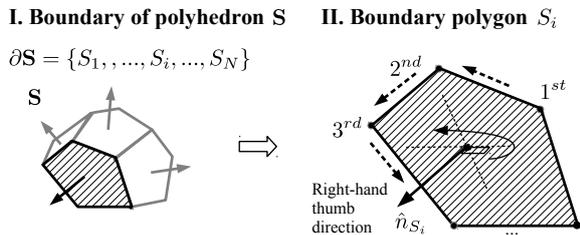
Figure 2: Example of a boundary representation (B-rep) of a building solid S.
