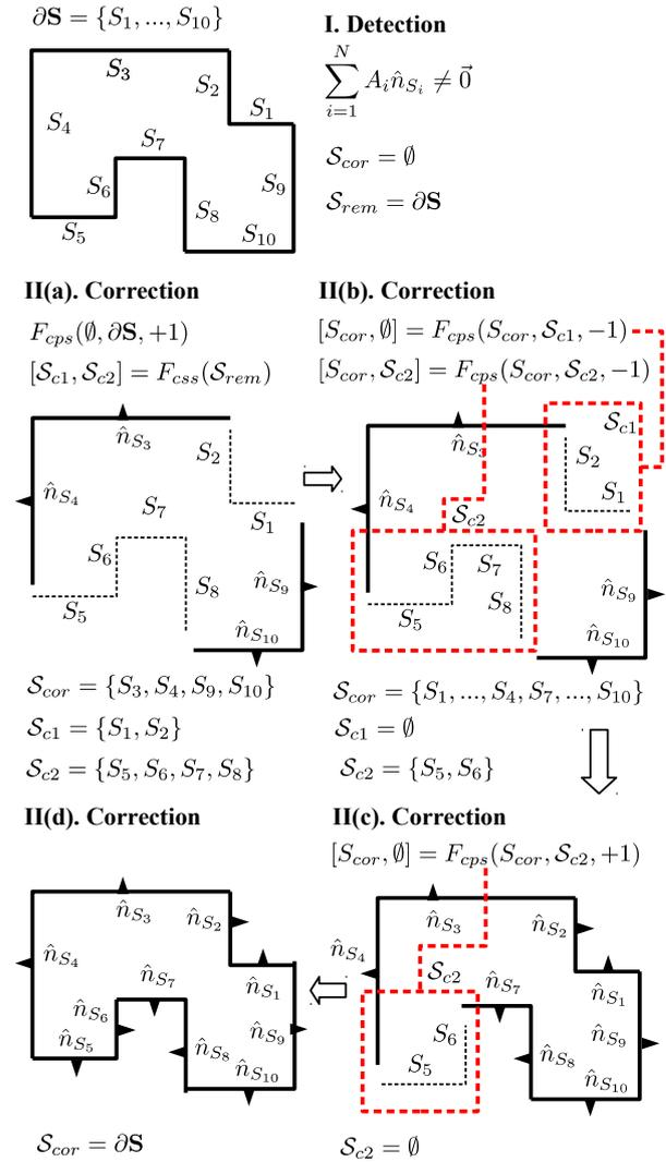
Figure 9: **Surface orientation errors detection and correction.** **I. Detection:** The vector sum of the surfaces does not add to zero. **II. Correction :** Convex hull normal corrections ( $F_{cps}$ ) and connected surface set partitioning ( $F_{css}$ ) are applied sequentially.
