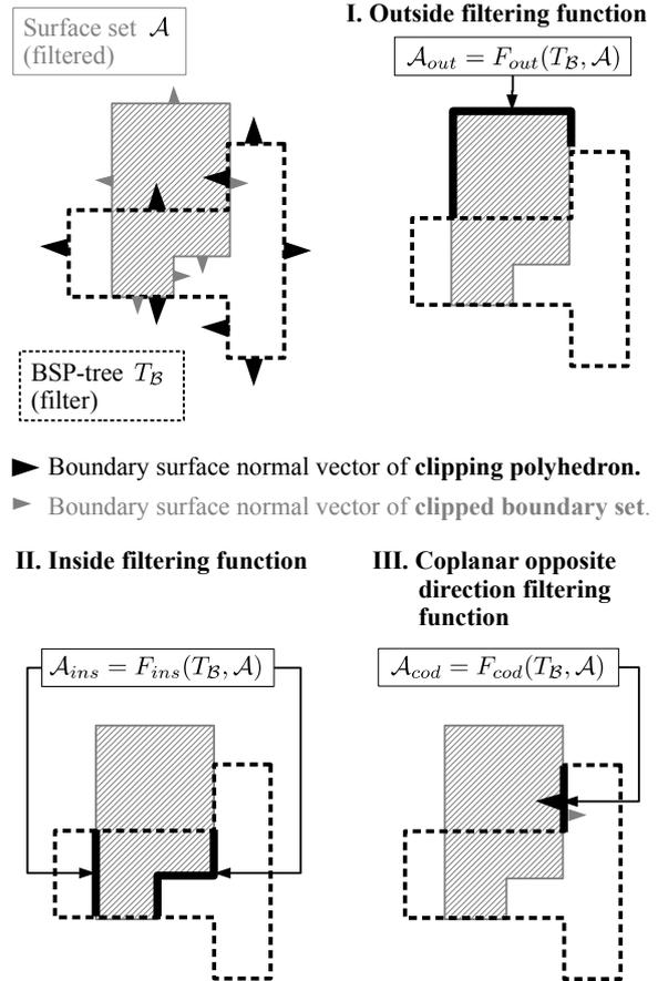
Figure 5: **I. Outside filtering function:**  $F_{out}$  returns parts of  $\mathcal{A}$  which lie outside  $\mathcal{B}$ , **II. Inside filtering function:**  $F_{ins}$  returns parts of  $\mathcal{A}$  which lie inside  $\mathcal{B}$ , **III. Coplanar opposite direction filtering function:**  $F_{cod}$  returns parts of  $\mathcal{A}$  which are coplanar with boundary surfaces of  $\mathcal{B}$  and have opposite normal vectors.
