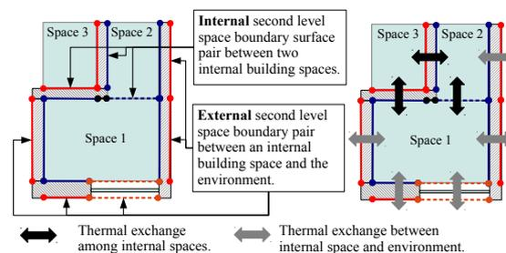
Figure 1: Example of second-level space boundary surface pairs
