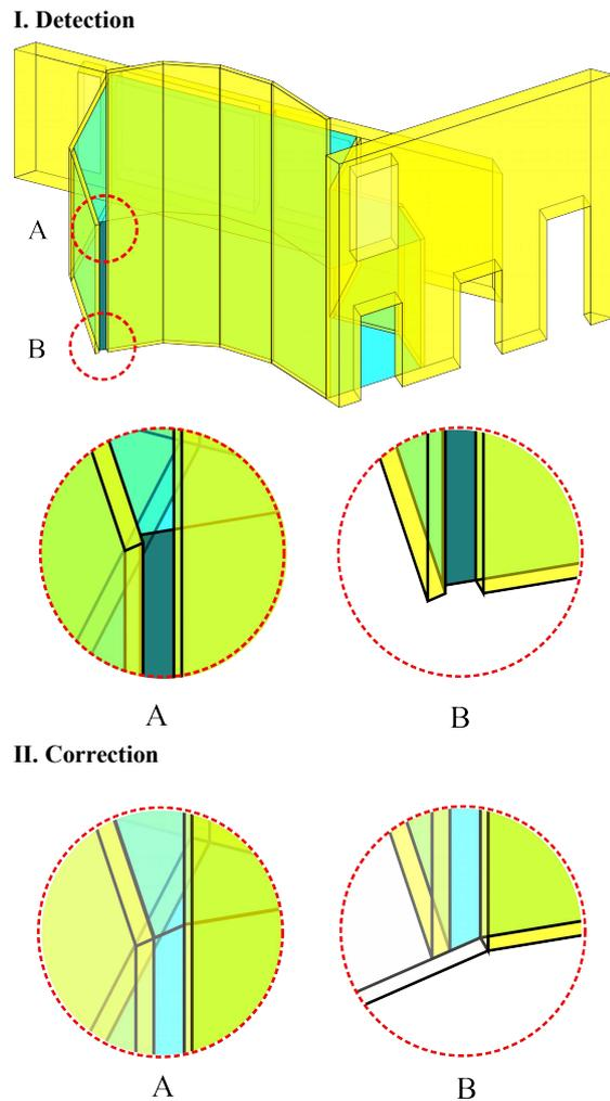
Figure 12: Space definition error example in TUC building: **detection (I)** and **correction (II)**.
