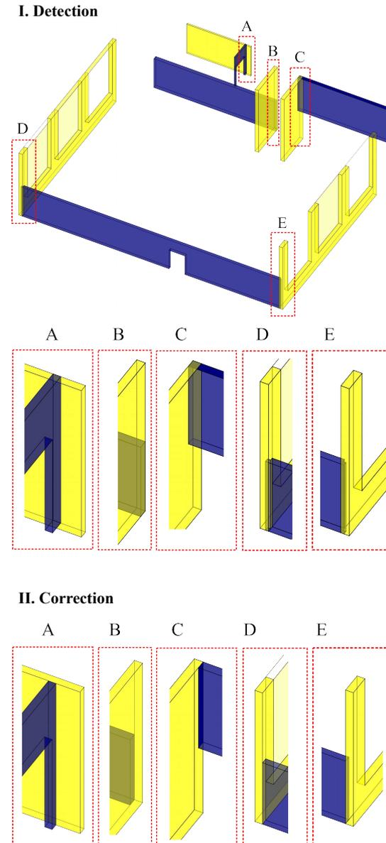
Figure 11: Wall-wall class error example in CARTIF building: **detection (I)** and **correction (II)**.
