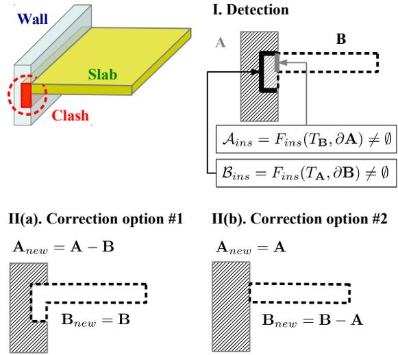
Figure 7: Clash error detection and correction. **I. Detection:** The surface sets returned by  $F_{ins}$  are nonempty. **II(b). Correction option #1:** **A** is replaced by  $\mathbf{A} - \mathbf{B}$ . **II(b). Correction option #2:** **B** is replaced by  $\mathbf{B} - \mathbf{A}$ .
