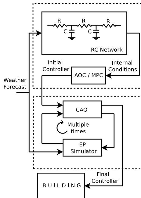
Fig. 7. Model-assisted control
