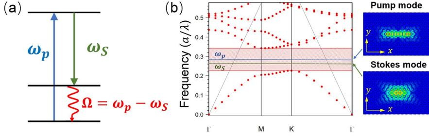
Fig. 2. (a) Schematic diagram of stimulated Raman scattering: a pump photon with frequency  $\omega_p$  interacts with a Raman-active optical medium and generates a Stokes photon with frequency  $\omega_s$  and a phonon with frequency  $\Omega = \omega_p - \omega_s$ . (b) Transverse-magnetic band structure of the photonic crystal and the two cavity modes. The field profile of the cavity modes are shown in the right panels.
