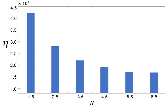
Fig. 4. The enhancement of the effective Raman susceptibility of the nonlinear metasurface relative to the intrinsic Raman susceptibility of silicon vs. the number of holes located along the  $x$ -direction between the end of the nanocavity and the boundary of the unit cell.
