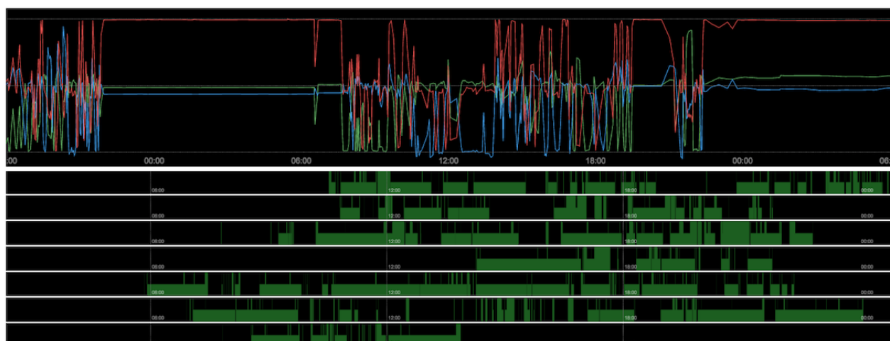
Figure 3. Two sample variables from the researcher-facing dashboard for a single participant. Upper panel: accelerometer output from smartphone showing periods of rest-activity over a continuous 36-hour period; lower panel: smartphone screen state showing screen doze state (lower bars) and active screen state (upper bars) over 7 days.
