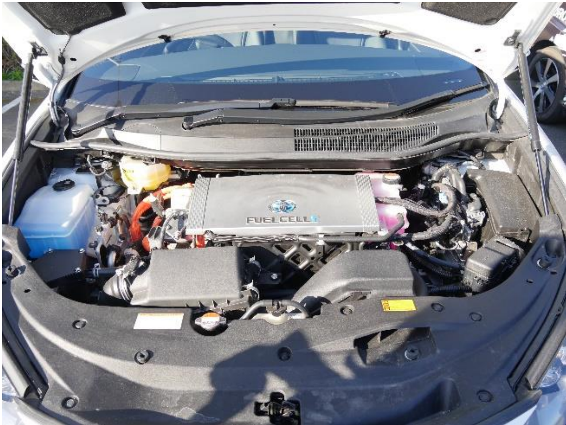
Figure 10. Front view of a FCEV, where the FC is in the middle
