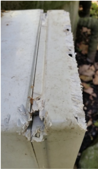
Figure 10: Air quality sensor after squirrel attack
