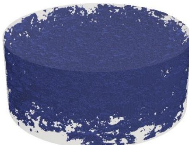
Fig. 2: Pore structure of ROI of 28-day old cement paste
