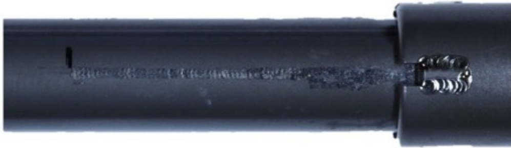
Figure 9. Image of Nail-7 (P2) showing relatively severe surface damage and wear occurring in a location corresponding to the position of an anti-rotation slot. In this implant, the anti-rotation slot seems to be intact with no visible sign of crack propagation.
