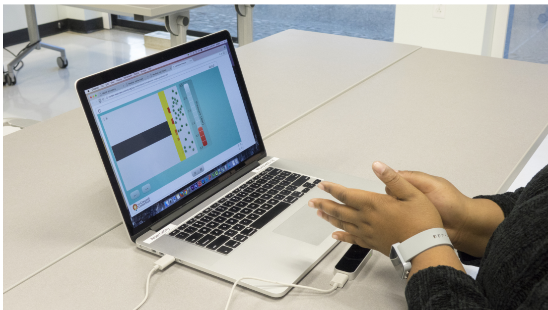
Figure 3. The GRASP simulation of air pressure where a user controls the simulation by representing the frequency by which the molecules are striking the surface of the container.
