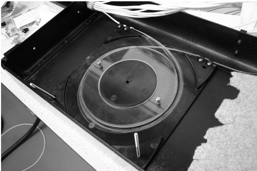
Figure 5: Fibre loop in the strain relief box. The Perspex template is removed after the loop has been laid.
