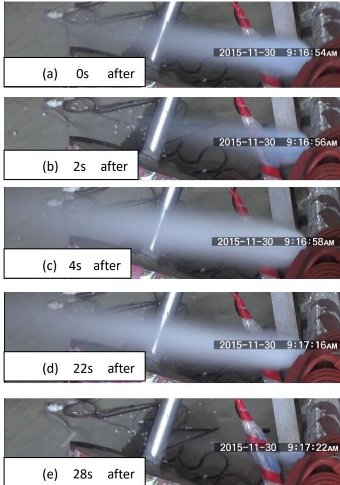
Figure 7 Jet flow phenomena (initial pressure of 9 MPa, initial temperature of 40 °C, and leakage hole diameter of 4 mm).
