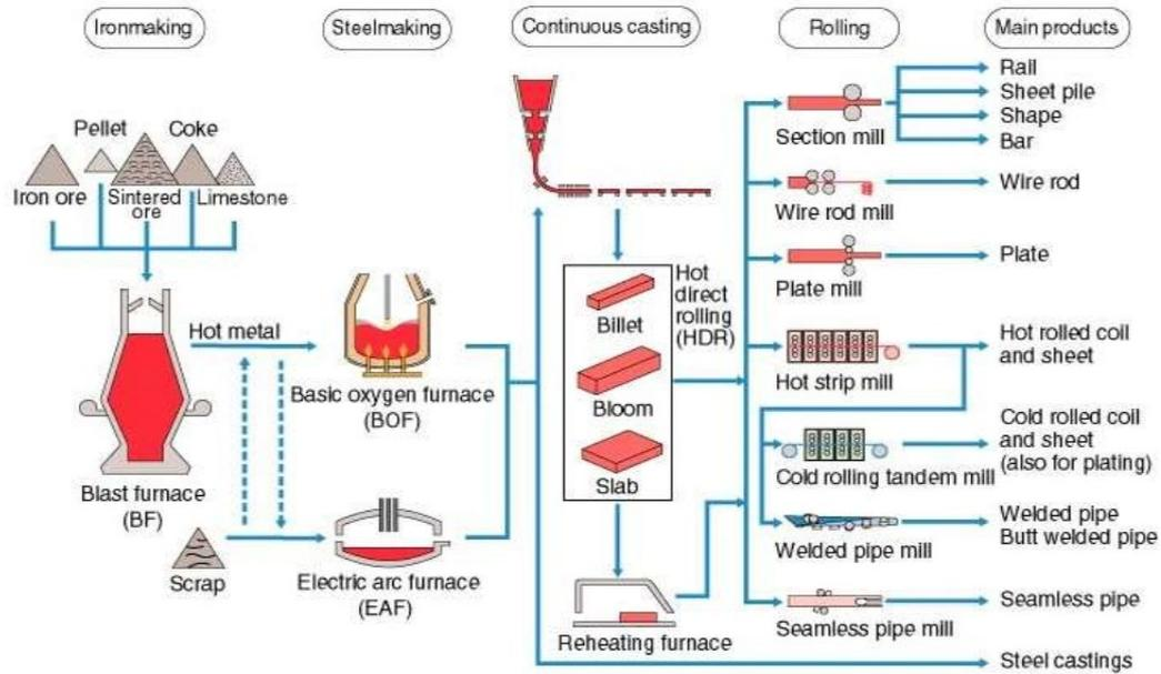
The manufacturing process of iron and steel to help the understandings.
