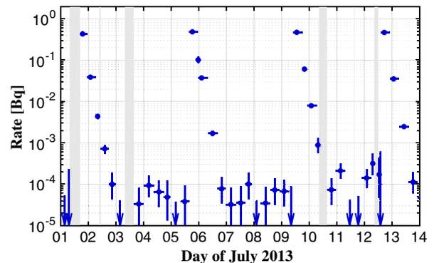
FIG. 3. The  $^{83\text{m}}\text{Kr}$  rate within a fiducial volume selection over a period of two weeks, during which four injections were performed. The dosing system is able to inject a small and repeatable activity. For small injections, it takes  $\sim 1$  d for the  $^{83\text{m}}\text{Kr}$  activity to fall below the baseline electron recoil background rate passing these selection criteria.
