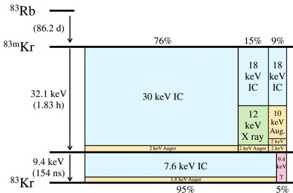
FIG. 1. Decay scheme of  $^{83\text{m}}\text{Kr}$ . The width of each column is proportional to the branching fraction of that decay mode, the vertical divisions are proportional to energy partitioning among internal conversion electrons (blue), Auger electrons (yellow), x rays (green), and gamma rays (red). Numerical values from Ref. [2].
