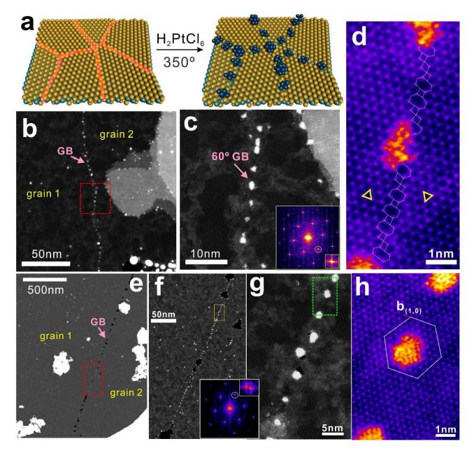
Figure 1. (a) Schematic illustration of decorating GBs of monolayer MoS<sub>2</sub> with Pt nanocrystals. (b) Low-mag ADF-STEM image showing the deposition of Pt nanocrystals on a APB. (c) Zoomed-in ADF-STEM image of
