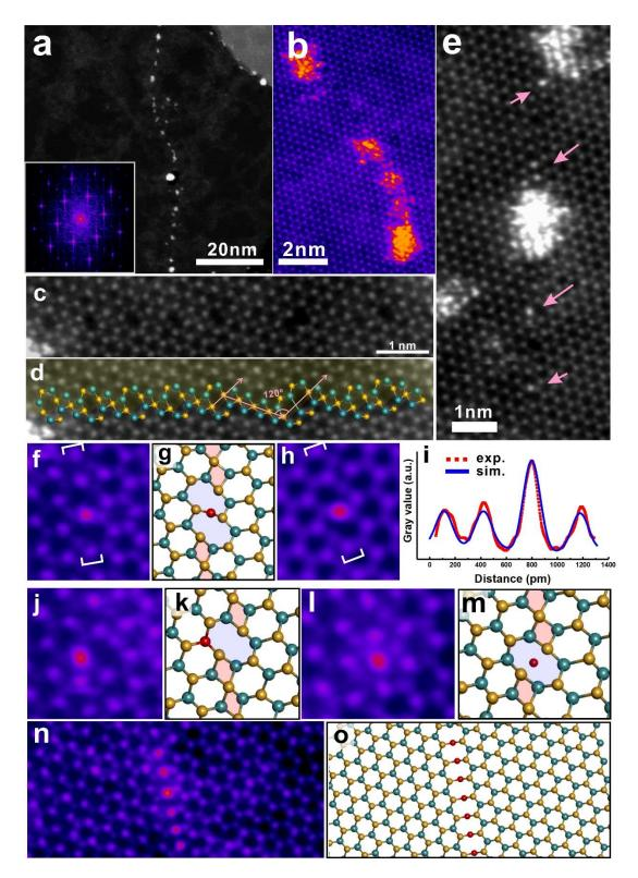
Figure 5. (a) Low-mag ADF-STEM image showing the decoration of Pt nanocrystals on a APB. Inset is the FFT of (a). (b) Medium-mag ADF-STEM image exhibiting the random and non-uniform attachment of Pt nanoparticles along the APB. (c) High-mag ADF-STEM image showing the atomic structure of the APB. (d) Overlay of atomic models of 4- and 8membered rings in a straight APB with the ADF-STEM image in (c), with a semi-transparent mask in yellow covered in
