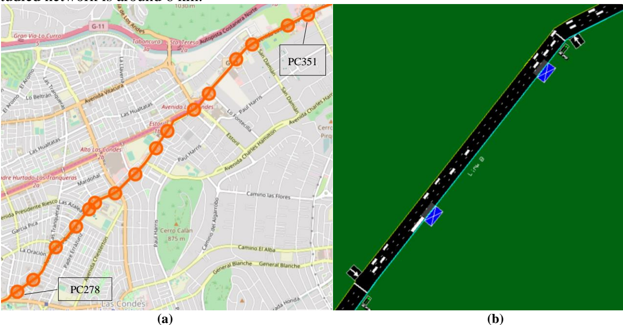
27 FIGURE 1 (a) Bus stops of bus route C01 along Avenida Las Condes and (b) simulation 28 model of part of the network when testing the effect of bus lanes
