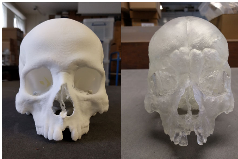
FIG. 4—3D printed cranium replicas, printed using SLS (left), SLA (right). [Color figure can be viewed at wileyonlinelibrary.com]
