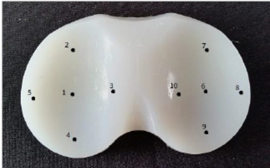
Figure 2. Image showing measurement points on CR type retrieved implant.
