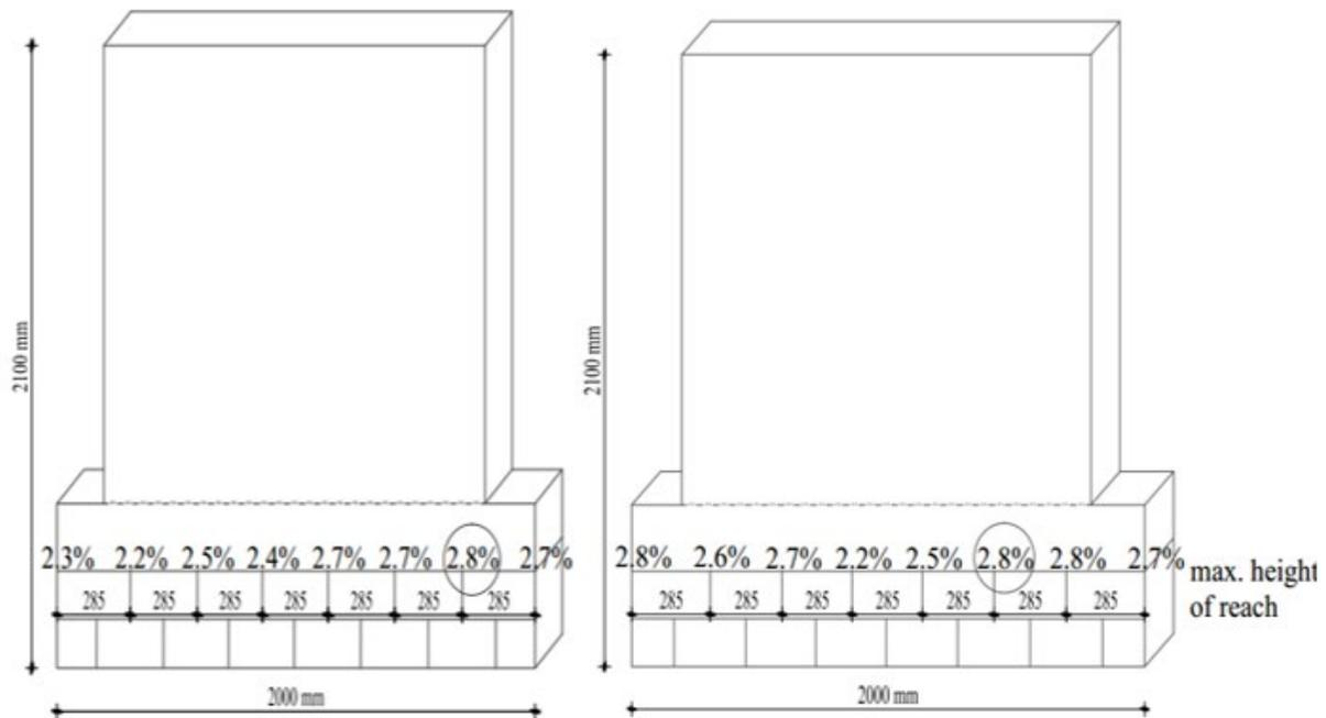
Fig 9 Schematic diagrams of the two walls with the various moisture contents as recorded by the moisture meter. (left-SB6 and right-CB6)
