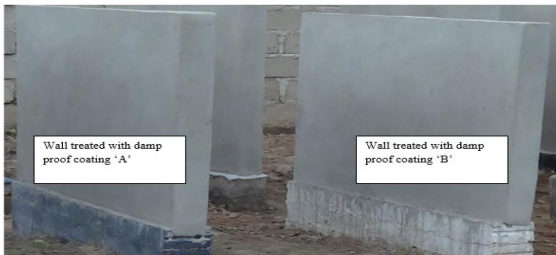
Fig 6 Photograph of test walls after they were treated with the damp proof coatings
