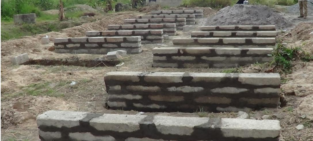
Fig 1 Photograph of test walls (extreme left are those constructed with SBs and extreme right are those constructed with CBs) (Source: Agyekum *et al.*, 2016)
