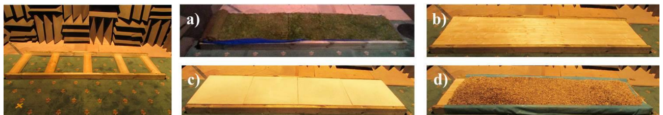
Figure 1 - The wooden platform used for the experiment on the left, covered in turn with the four selected materials: a) Grass, b) Wood, c) Stone, and d) Gravel
