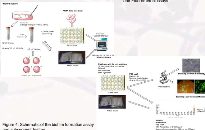
Figure 4: Schematic of the biofilm formation assay and subsequent testing.
