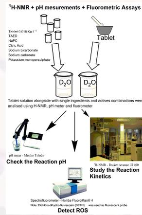
Figure 3: Schematic of H-NMR, pH measurements and Fluorometric assays
