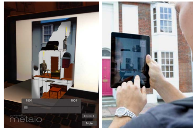
Figure 1: First AR prototype. Figure 2: AR Experience: by pointing the mobile device to a predefined façade the digital content appears superimposed on the façade.
