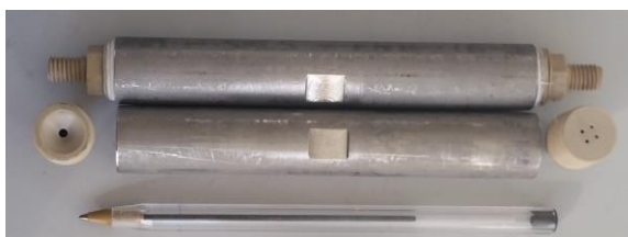
Figure B-1: Individual cells (~18.75 mL) for the RotaChrom CPC.
