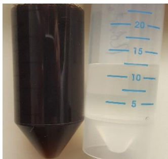
Figure 6-14: Visual comparison of the crude hydrolysate (left) and the decolourised crude hydrolysate (right). Decolourisation was performed as described in Section 2.15.2.
