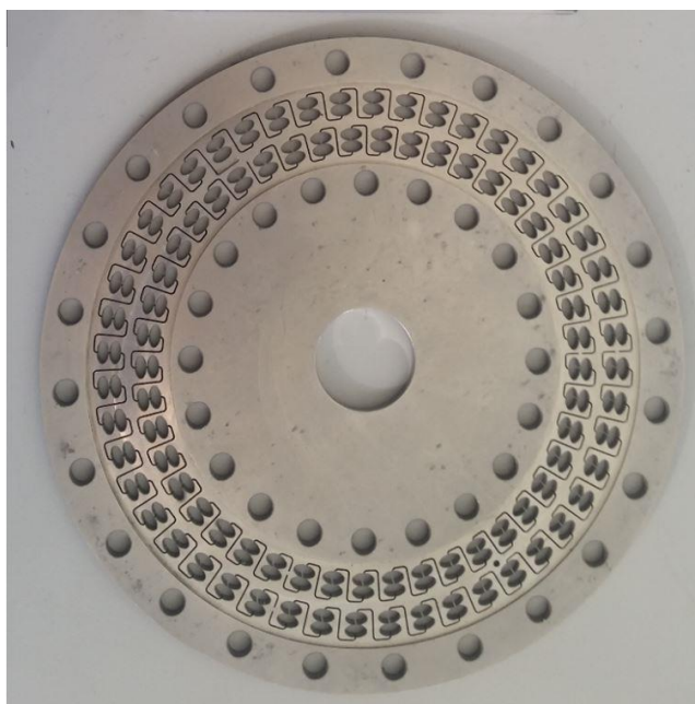
Figure 1-6: Individual disk (~6.7 cm radius) from an Armen CPC machine (Vannes, France) featuring a twin cell design.
