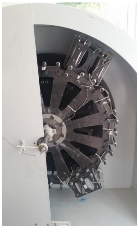
Figure B-2: RotaChrom rCPC with two cell stacks containing 32 cells each.
