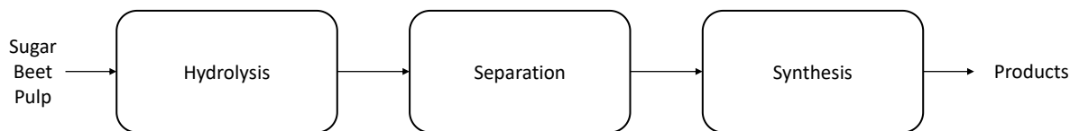
Figure 1-3: Schematic process overview for producing sustainable chemical feedstocks from sugar beet pulp.
