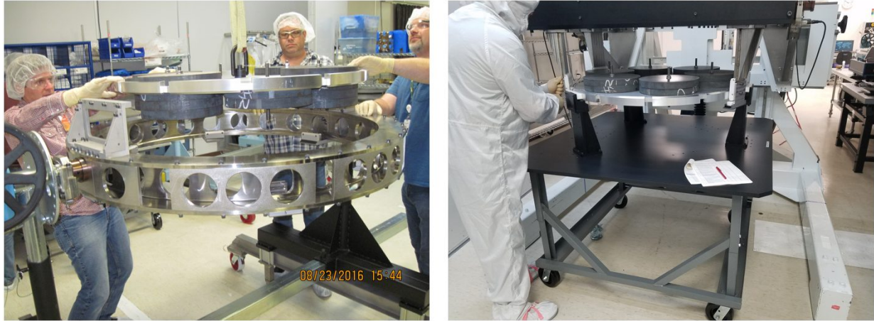
Figure 4. Load testing coating fixture to 1.5 times maximum lens weight using metal mass surrogate is shown on left. Weights were added to increase weight as needed. Testing was completed at 431 kg, 1.5 times the weight of the heaviest lens, C4. Practice and test procedures with full weight metal C4 surrogate is shown on right. The operation shown is practice moving the lens to a mobile transfer table from the shipping crate.
