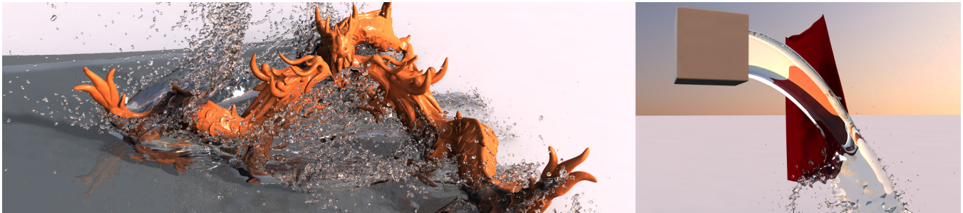
Figure 1: Left: Breaking dam scenario with 1.94 million particles, featuring obstacles with complex solid boundaries. Right: Fluid and cloth are simulated together in the Projective Dynamics framework.
