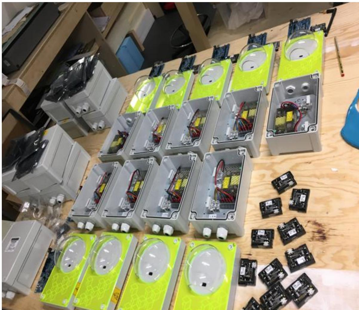
**Figure 4** ICRI Environmental Sensor Assemblies.
