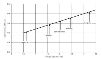
Figure 1: Relationship between built form and heat loss (from Steemers, 2003).
