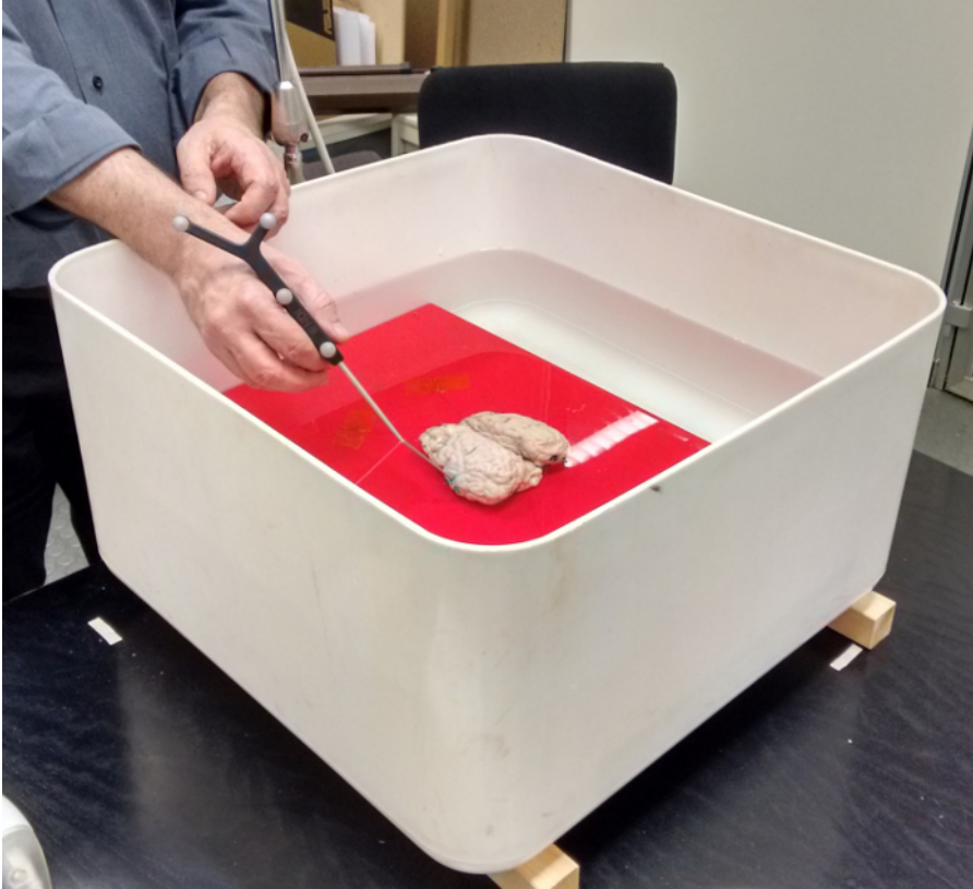
Figure 16: Acquisition of the positions of the glass spheres implanted in the bovine brain for calibration. The pointer tool tip is used to acquire, one by one, the positions of the 18 glass spheres implanted into the bovine brain immersed in water. These positions are used to compute the transformation from the motion tracking system space to the MR image space. Please click here to view a larger version of this figure.
