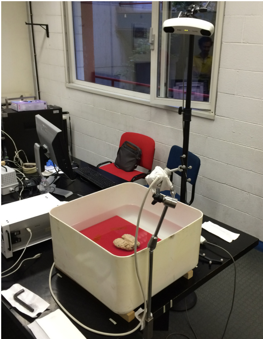
Figure 11: Setup of the experimental acquisitions with the motion tracking system. The motion tracking sensor is placed above the water tank in which the bovine brain is immersed, so that the target and the probe with the clamped reflecting markers entirely fit within its measurement field of view. Please click here to view a larger version of this figure.
