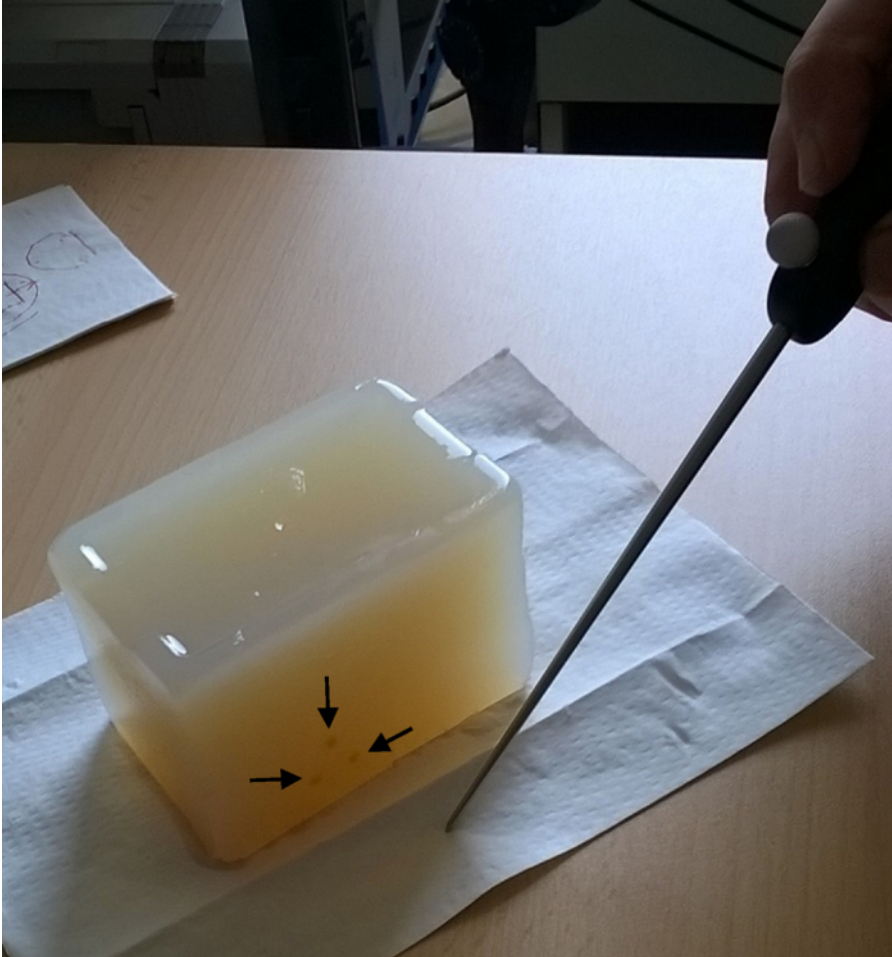
Figure 6: Agar phantom. The figure shows the agar phantom, in which an implanted pattern of three yellow-painted glass spheres (indicated by the black arrows) is clearly visible in the lower edge. The pointer tool tip, used to measure the sphere positions during the calibration phase, is also shown near the phantom. Please click here to view a larger version of this figure.
