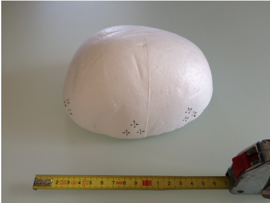
Figure 5: Polystyrene model of the brain used during the preliminary design stage. The polystyrene mannequin head, properly cut to mimic the bovine brain dimensions, was used to choose the positioning of the glass sphere patterns in the brain. Six triangular patterns of spheres, with a 3-mm diameter, have been implanted in the polystyrene model as shown in the picture, i.e. three patterns on the right and three on the left brain hemispheres. Please click here to view a larger version of this figure.
