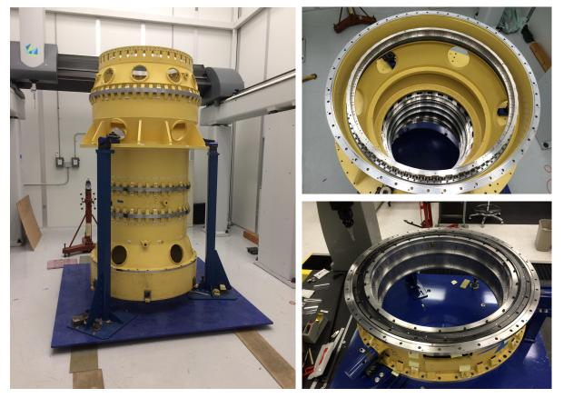
Figure 3. Fully assembled DESI corrector barrel in the Fermilab CMM used for the alignment (left), a view of the lens cells inside the barrel (upper right) and a picture of the Middle section showing the lens cells that support the ADC lenses and the bearings that is used to rotate the lenses (lower right). The yellow color is just the temporary primer, after all the work was finished the barrel was painted with black Aeroglaze Z306.
