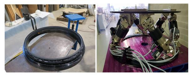
Figure 5. The picture on the left shows one of the two ADC rotator bearing and gear segments. The outer race of the bearings attaches to the Middle section and the inner race to the ADC lens cell. The gear is driven by a harmonic drive mounted to the outside of the Middle section. The picture on the right shows the final assembly of the hexapod at A.D.S International LLC.
