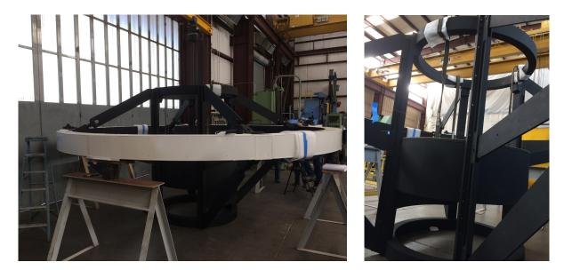
Figure 7. The left picture shows the Upper Ring, Vanes and Cage as-built structure at CAID Industries in Tucson, Arizona. The picture on the right shows a detail of the Cage and how the vanes insert on the cage's rails.
